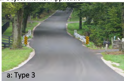
Figure 2: Object Marker Application
