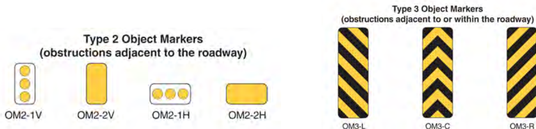
Figure 1: MUTCD Object Marker
