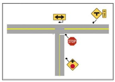
traffic control signs like stop ahead signing (W3-1) should be used. For intersections with persistent crash history or demonstrated high frequency/high severity of crashes, dual mounted signing may be utilized.
